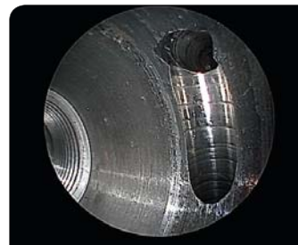
Inspection of a drill hole intersection for ensuring it is burr-free
