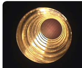
Well cut inner threads in hollow shaft for precision clocks
