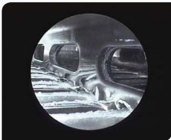
Checking the position of the intersection of two holes in a heat exchanger
