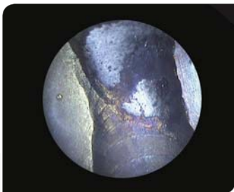
Run-out of a welded seam
