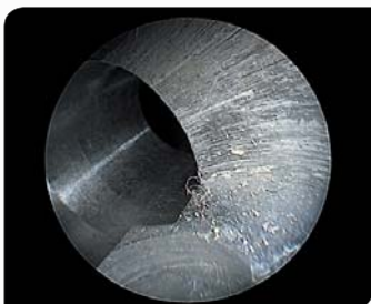
Inspection of a drill hole for ensuring it is burr-free
