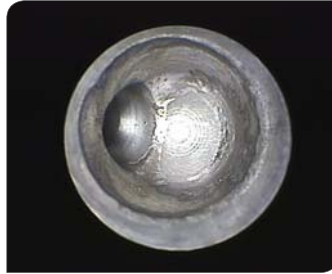
Examination of position and deburring in a nozzle body in the production process
